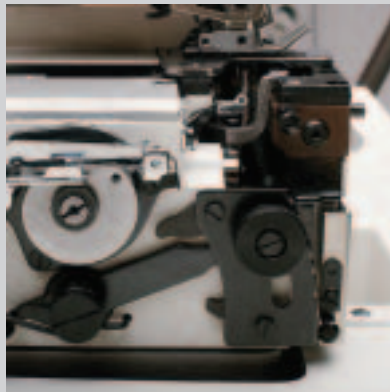
Differenzialtransportschnellverstellung Quick-change differential feed
