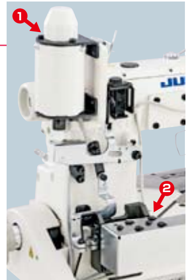
① Presser foot lifter drive mechanism magnet ② Thread trimmer drive mechanism magnet
