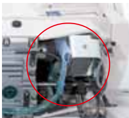
One-touch type reverse feed device
